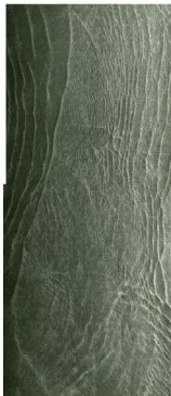
Figure 6. (Right) ERS-2 (C-band, VV) SAR image of the Andaman acquired on 11 February 1997 at 0338 UTC (orbit 8477, frames 3357, 3373, 3389, 3341, 3429, 3447, 3463, 3483, and 3501). The image shows a large number of internal wave packets and associated soliton-soliton interactions. Imaged area is 100 km x 900 km. (Below) An enlargement highlighting a middle portion of the image. Imaged area 235 km x 100 km ©ESA 1997.
